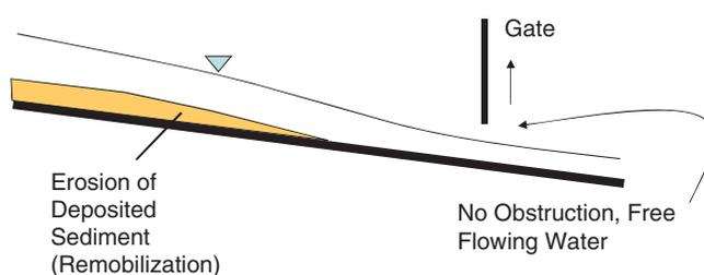
**Figure 8.** Schematic representation of drawdown flushing.
