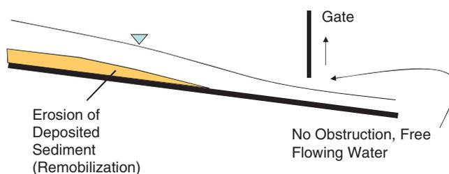
**Figure 8.** Schematic representation of drawdown flushing.
