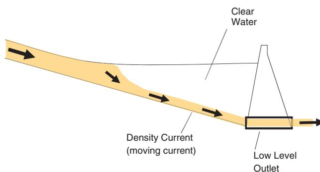
**Figure 14.** Schematic representation of density current venting.
