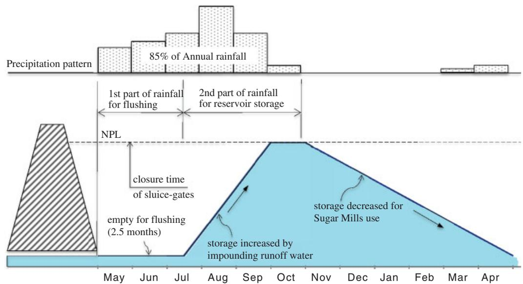
**Figure 11.** Seasonal operation of Jen-San-Pei reservoir in Taiwan to pass sediment. The reservoir was drawn completely down and the outlets left open for the first 2.5 months of the rainy season, to allow inflowing high flows to transport their sediment through the reservoir and scour sediment already deposited. Midway through the rainy season, the outlet gates were closed, so the reservoir could impound water to process sugar cane, harvested from November to April. [Redrawn from Huang, 1994]
