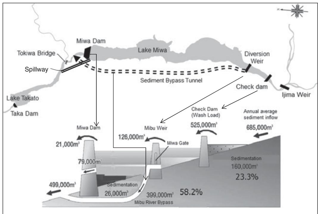
**Figure 3.** Diagram of sediment bypass system for Miwa Dam, Mibu River, Japan. A check dam traps coarse sediment, and a diversion weir diverts flows with high suspended sediment concentrations into a bypass tunnel.
