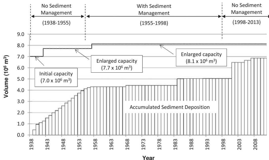
**Figure 10.** Deposition within Jen-San-Pei reservoir in Taiwan, 1938 to present. Prior to 1955, no sediment management was conducted and the reservoir filled rapidly, but beginning 1955 seasonal drawdown and sediment passing maintained reservoir capacity. From 1998 to 2012, the pass-through operations were stopped, allowing sediment to accumulate. Pass-through operation was resumed in 2013. [Modified from Huang, 1994 and extended to present using data from Water Resources Agency of Taiwan]
