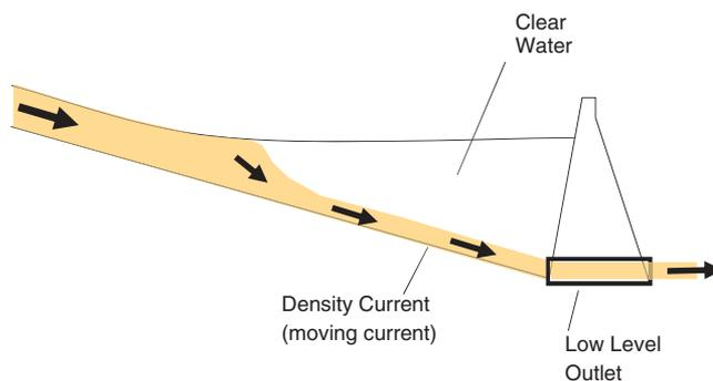
**Figure 14.** Schematic representation of density current venting.
