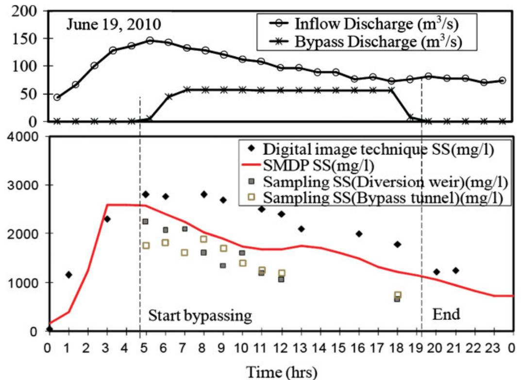
**Figure 4.** Sediment bypass at Miwa Dam June 19, 2010: (a) hydrographs for inflow into the reservoir and for flow through the bypass tunnel, and (b) suspended sediment concentrations (mg/l) at the diversion weir and in the bypass tunnel. [Modified from Kantoush et al., 2011]
