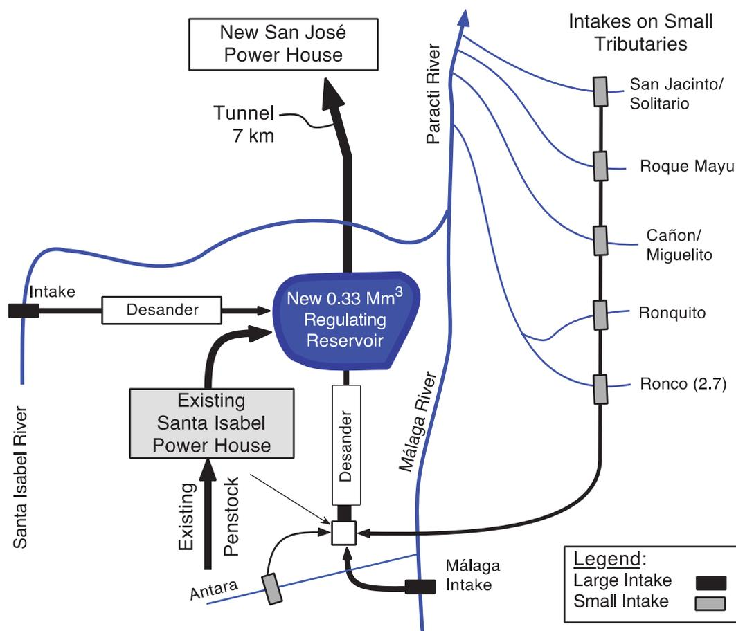
**Figure 5.** Schematic layout of 125 MW San José hydroelectric project, Paractia River, Bolivia, incorporating an off-stream regulating reservoir for pondage and desanders to remove the coarse sediment abundant in the streams.
