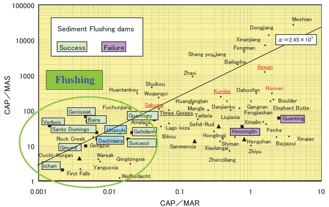
**Figure 9.** Plot of flushing projects from diverse environments showing that successful cases are characterized by impoundment ratios of 0.4 or less. That is, reservoir storage capacity divided by mean annual runoff (inflow to the reservoir) should be less than 0.4.
