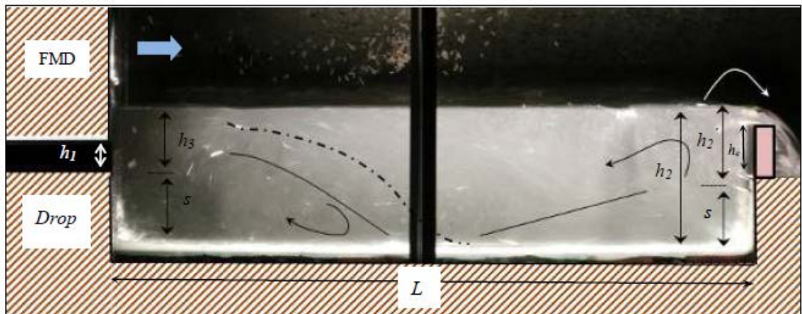
Figure 2 The conceptual schematic view for the problematic of a conventional stilling basin.
