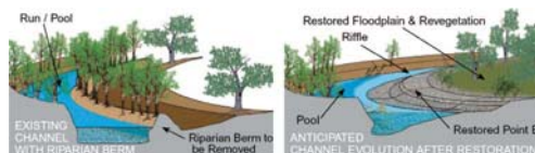
Figure 10. Sketch of channel rehabilitation. (McBain & Trush, Inc. 2000).
