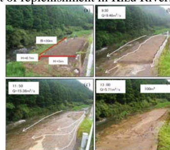
Figure 3. Evolution of sediment replenishment experiment in Kizu river[Kantoush et al. 2010]
