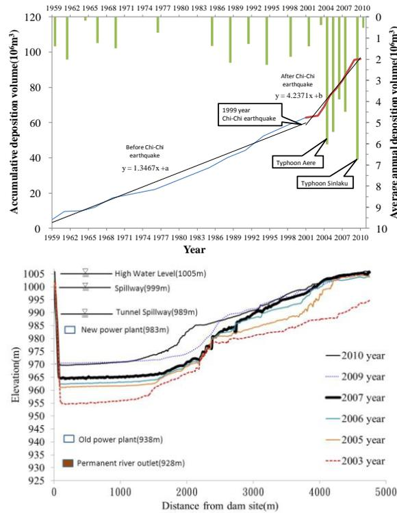
**Figure 3.** Variation of sedimentation in Wushe reservoir
