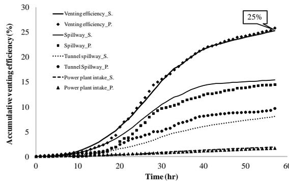
**Figure 10.** Experimental area with outflow structures of physical model **Figure 11.** Venting efficiency of existed facilities
