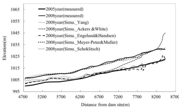
Figure 12. Verification of 1D numerical model at upstream river
