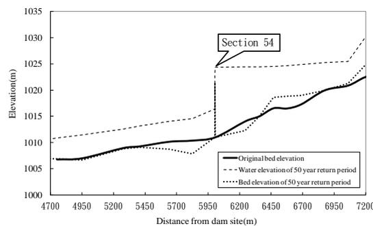
Figure 14. Water elevation and bed elevation after bypass operation of designed flood
