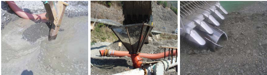
(A) Under water (B) Cast into the hopper (C) Direct suction Figure 7. Methods of suction tests.
