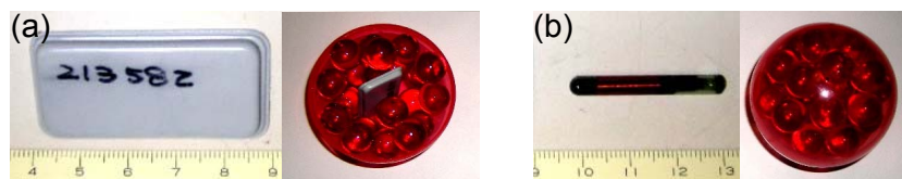
Figure 3 (a) RUBEE- Tag (50mm×25mm, 3mm), (b) Passive TI-RFID( \phi 3.85mm 32mm)
