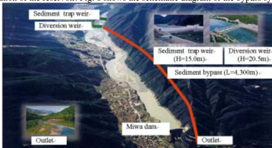
Fig. 6 Sediment Bypass Scheme at Miwa Dam
