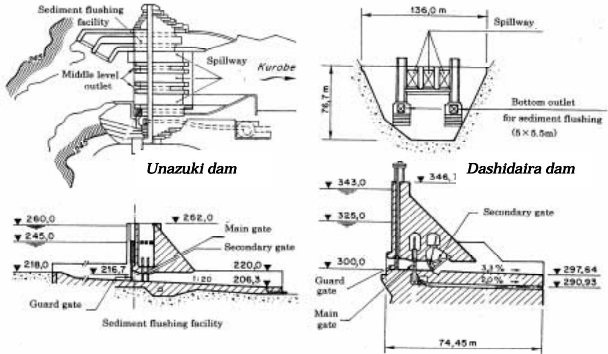
Figure 14. Schematic diagram of the Unazuki dam(left) and the Dashidaira dam(right)
