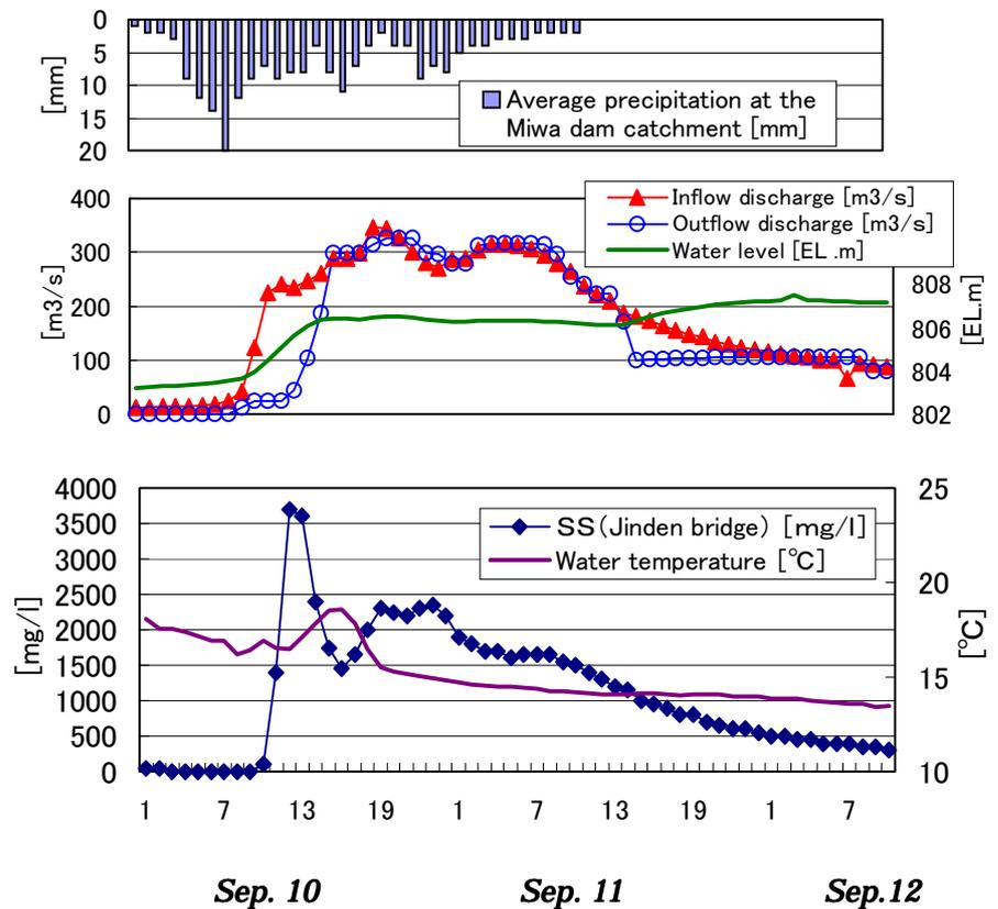
**Figure 11. Field experiment at the Miwa dam 'Typhoon No.15, 2001'**
