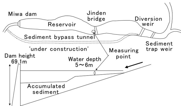
**Figure 8. Field experiment of the submersible type SMDP at Miwa dam**
