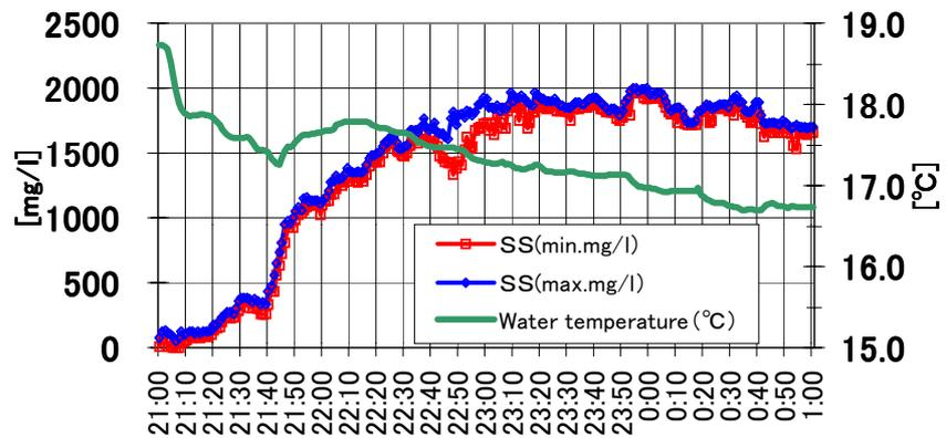
**Figure 10. SS and water temperature change in every minute 'Typhoon No.11'**
