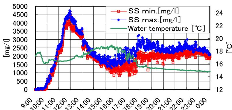
**Figure 12. SS and water temperature change in every minute ‘Typhoon No.15’**
