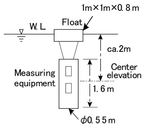
**Figure 3. Schematic diagram of the submersible type SMDP**
