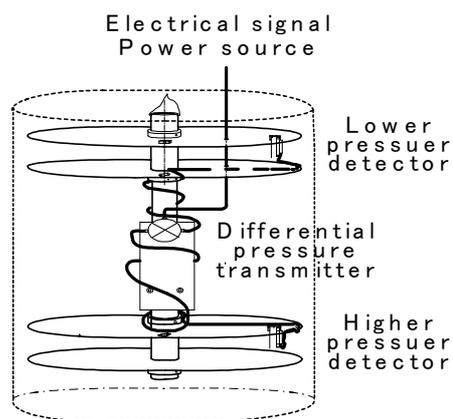
**Figure 2. Schematic diagram of the measuring equipment**
