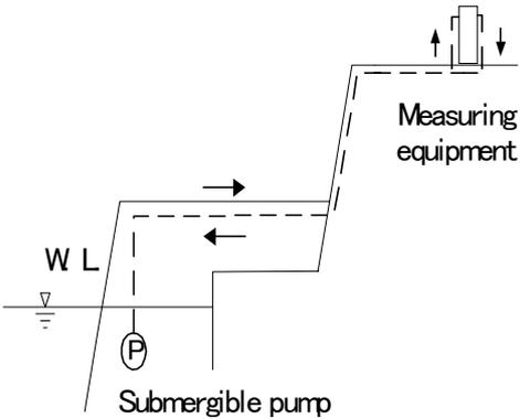
**Figure 5. Schematic diagram of the water circulation type SMDP**
