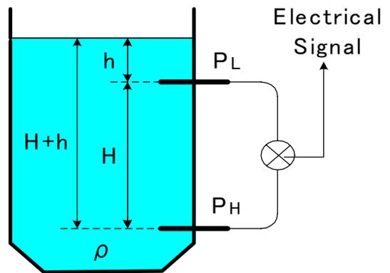
**Figure 1. Measuring principle**
