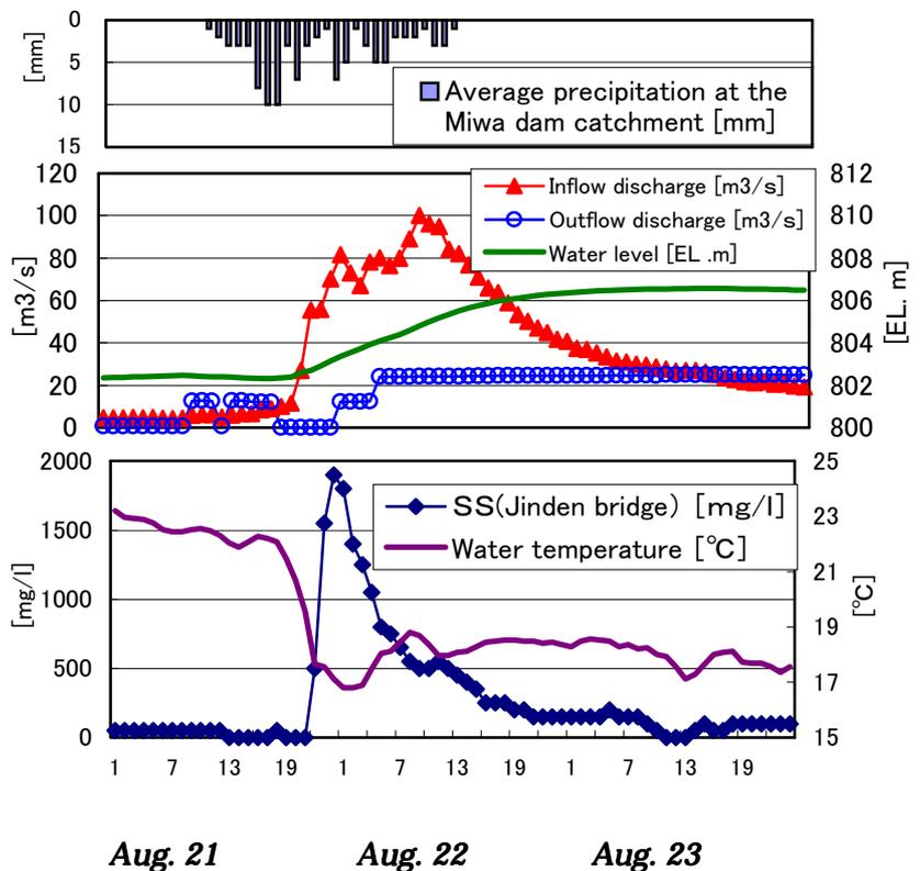
**Figure 9. Field experiment at the Miwa dam 'Typhoon No.11, 2001'**
