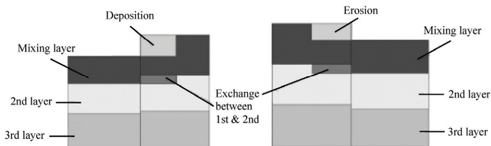
Fig. 19 Multiple-layer sorting model of bed material gradation
