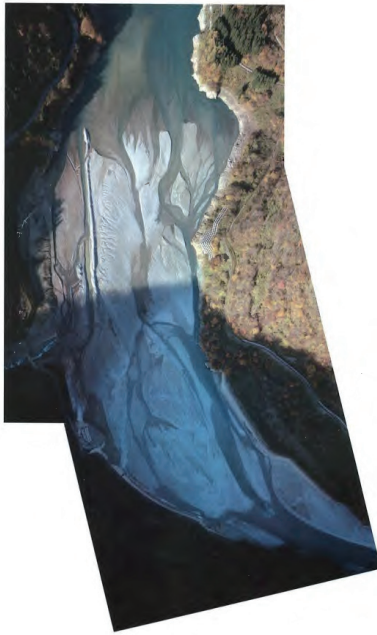
Fig. 6. Aerial photo showing the irregular scouring channels after the flushing operation in the study zone of Unazuki reservoir (Photo provided by the Kurobe Office of River).
