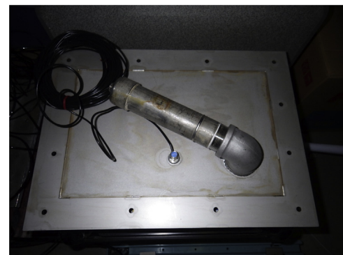
Fig. 3. Back side of the impact plate, the smaller sensor represents the acceleration sensor and the microphone is in the steel pipe (courtesy of Hydrotech Co., Ltd.).
