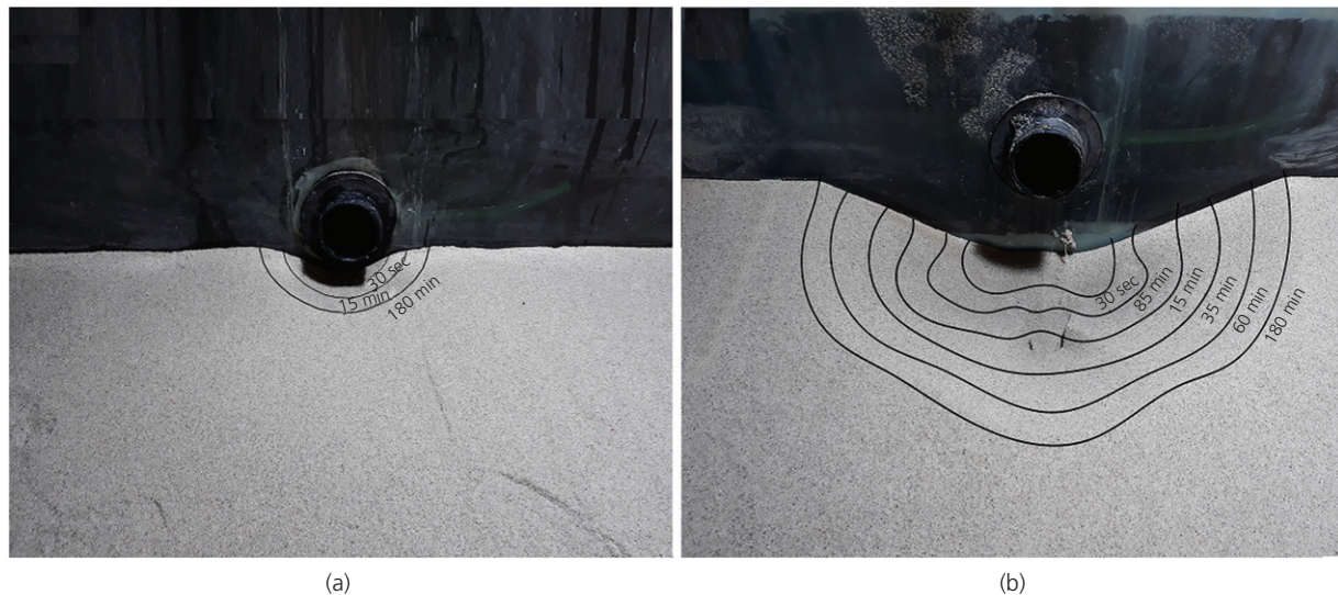
Figure 12. The development pattern of flushing cone with time in (a) non-structural and (b) structural test
