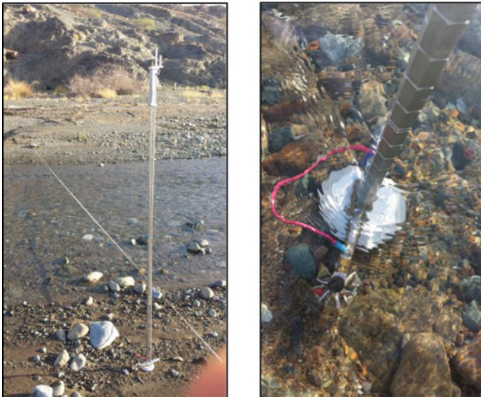
Fig. 9.3 Current meter measurement method
