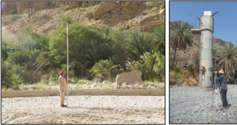
Fig. 9.2 Slope-area method using levelling instruments
